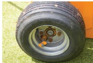
Simple “pull & twist” clutch levers on each wheel to disengage wheel drive to the brush during transport
