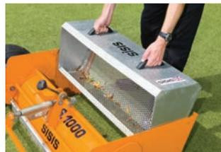
Easy to remove hopper and unwanted debris
