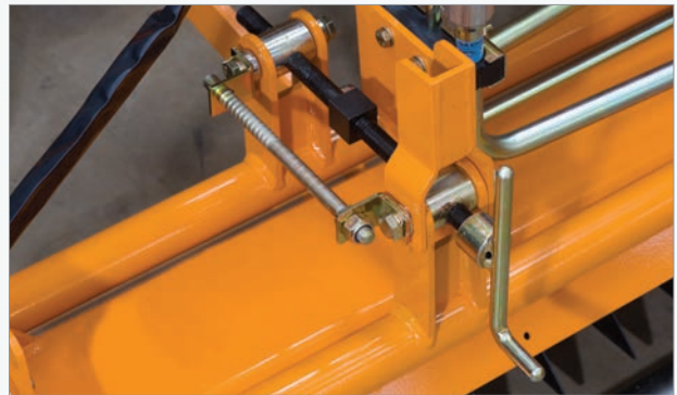
Micro adjusters for depth setting
