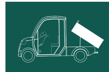
Electric tilt cargo bed with removable drop sides. L. 1258 x B. 1215 x H. 300 mm
