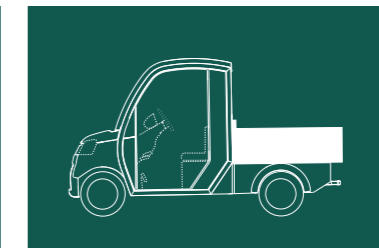
Cargo bed with removable drop sides. L. 1258 x B. 1215 x H. 300 mm
