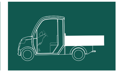
Cargo bed with removable drop sides. L. 1618 x B. 1215 x H. 300 mm**
