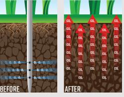
FORCES OXYGEN IN AND PUSHES CO<sub>2</sub> AND OTHER ANAEROBIC GASES OUT FOR IMPROVED ROOT ZONE GAS EXCHANGE
