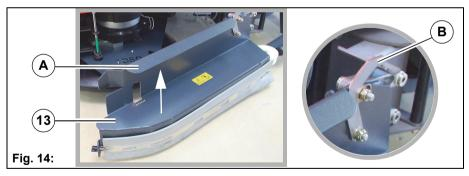
The wipers can be raised if necessary. To do this, raise the wiper at the handle **Fig. 14-A** and hook the locking hook **Fig. 14-B** into the bracket above it.
