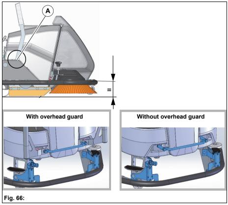
If the pre-sweep suction unit is attached to the machine and the lever is in the sweeping position (Pos. 1) **Fig. 65-A**, the frame must be aligned parallel to the floor.
