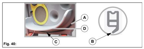
Check the function of the seal in the tank cap **Fig. 40-A** daily and replace it if damaged.
