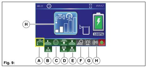
The soft keys are selected by rotating the turn-push knob (soft key with yellow border) and confirmed by pressing. An action window **Fig. 9-H** opens, in which the settings can be carried out using the turn-push knob. The action windows close automatically after a few seconds or by pressing the return key.
