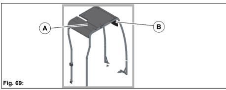
The overhead guard **Fig. 69-A** is used to protect the driver from falling parts in the high bay warehouse, for example.
